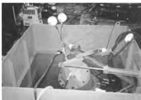
Photo. 3 Durability test of Universal joint
